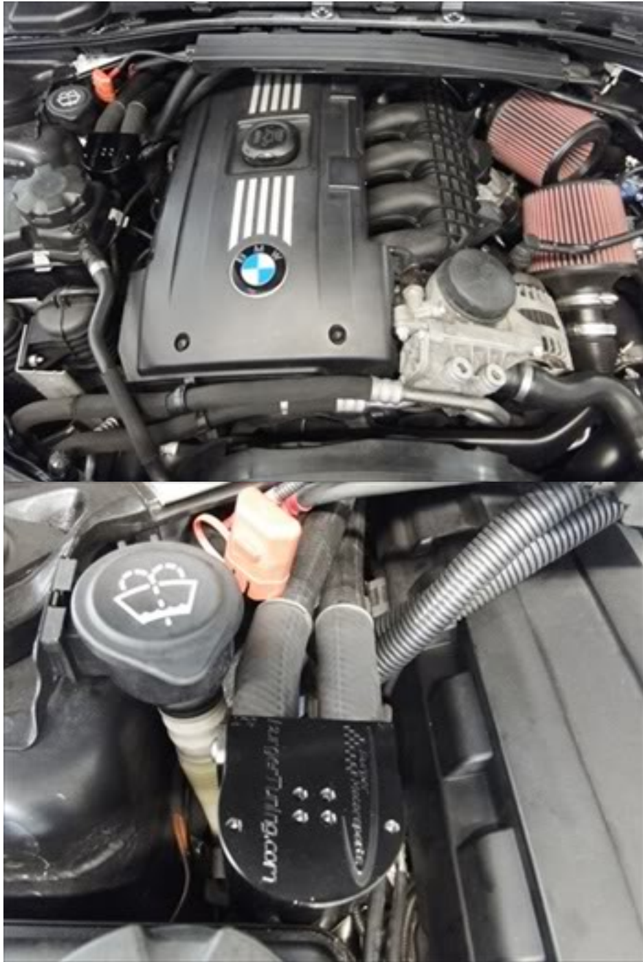
Pic Below: Attaching the Can in this way will prevent it from rattling during driving. Drilling on the body of the 335 is not necessary since there is already a small screw that you can attach the Can plate against.
